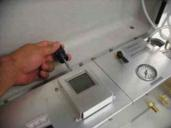
12. Connect the charger to the unit to charge the battery before collecting a sample. The fast-charge light on the charger goes out when the battery is fully charged. Charging may take up to 12 hours.
