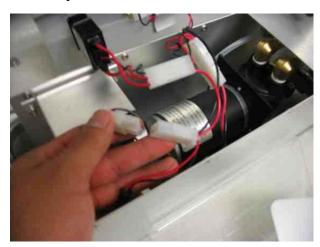
5. Remove the 2 battery hold-down nuts using a 5/16" wrench, then remove the hold-down bracket.
