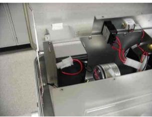
6. Remove the old lead-acid battery. Do not remove the wires and connector attached to battery.
