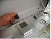
4. Disconnect battery from the unit's circuitry.
