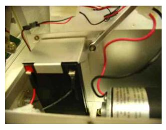
7. Set the new lead-acid battery in place. Note that the new battery includes wires and connector.
